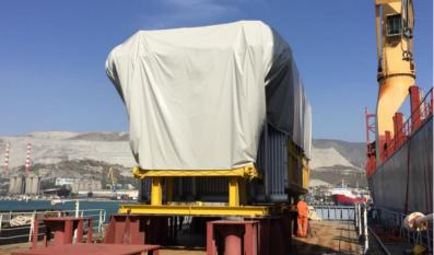
Ocean transportation of 1x Steam Turbine weighting 140 tons (4.8 meters height) + 1 x Generator weighting 95 tons from Marina di Carrara + Immingham to Haifa, discharging and delivery by road up to Hadera, Israel (GE O&G for Hadera power plant).
