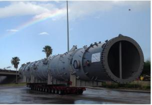
Multimodal transportation of 1 x Boiler weighting 145 tons (5.5 meters high) to Porto Marghera including road transport from Manufacturer to Valdaro river port, direct transshipment from trailer to barge, river transport from Valdaro to Porto Marghera, discharging onto trailer and FAS delivery.
