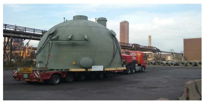
Door to door delivery of 1 x Transfomer weighting 175 tons from North Italy to Tullahoma, TN including road transportation up to Marghera port, loading onto vessel, ocean transportation from Porto Marghera to Mobile, discharging and combined rail + road delivery up to Tullahoma, TN (Final Client: Arnold AFB).
