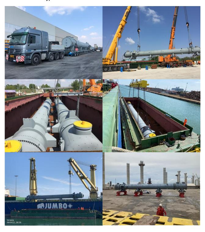
Multimodal transportation up to Porto Marghera (road trailer + river barge), loading onto vessel and ocean transportation from Porto Marghera to Freeport port of 1 x Reactor measuring 31.0 x  $5.4 \times 5.7$  m and weighting 155 tons (Final Client: Olin Corporation Plant).
