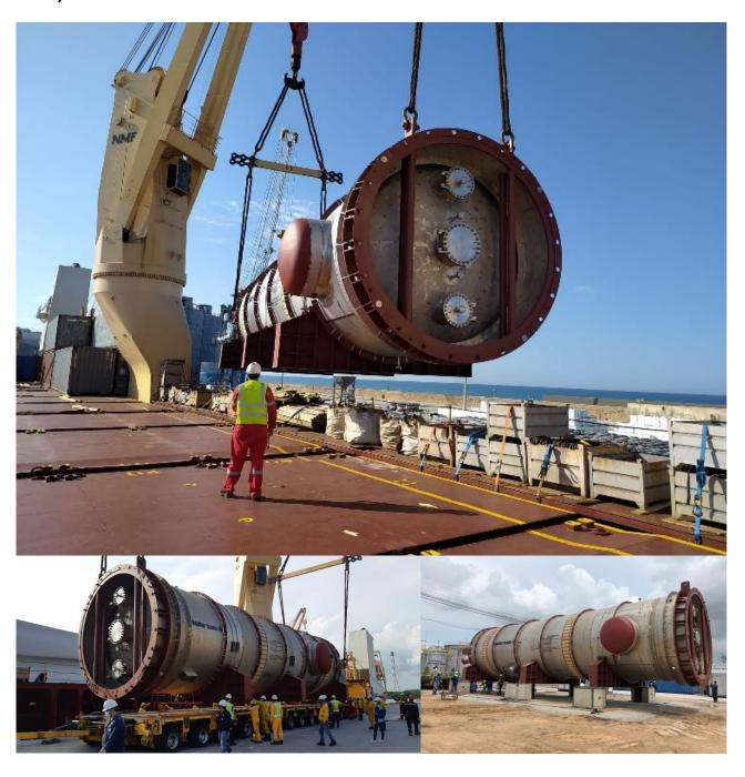
Door to door delivery of 2 x Exchanger (28 meters long and weighting 153 tons each) from Cremona to Corpus Christi, TX including multimodal transportation up to Porto Marghera (road trailer + river barge), loading onto vessel, sea transportation from Porto Marghera to Corpus Christi port, discharging and road delivery up to job site (Final Client: Flint Hills Resources Refinery).
