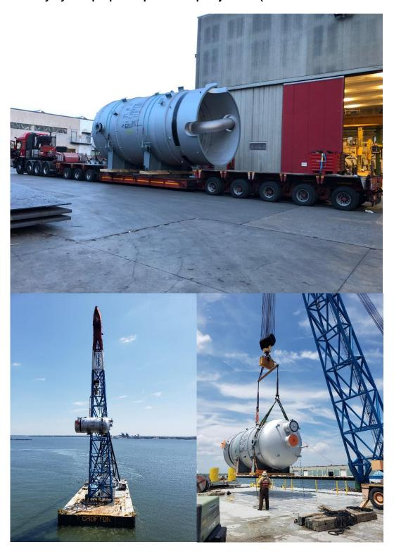
Road transportation from construction yard in Jebel Ali to loading jetty, loading onto vessel and ocean transportation of 1 x Exchanger (measuring 56.5 x 7.4 x 9.0 m and weighting 1650 tons) from Jebel Ali to Guangzhou, by chartering of suitable super heavy lift vessel (Final Client: China Petroleum).
