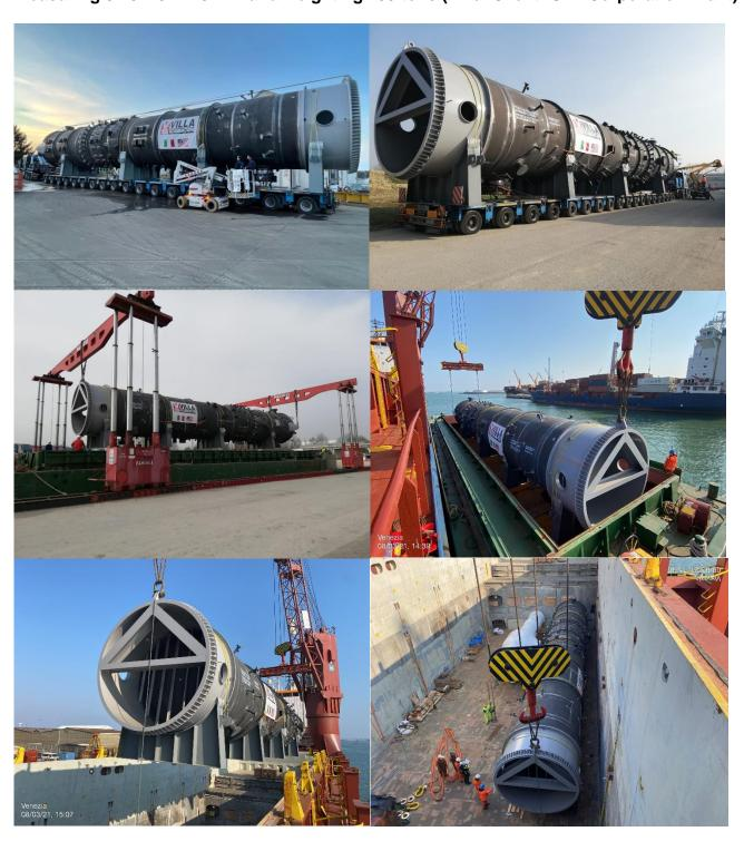
Door to door delivery of 1 x Reactor (19 meters long and weighting 84 tons) + 1 x Reactor (28 meters long and weighting 43 tons) from Massa to Port Arthur, TX including road transportation up to Marina di Carrara port, loading onto vessel, ocean transportation from Porto Marghera to Port Arthur, discharging and road delivery up to job site (Final Client: Valero Refinery).
