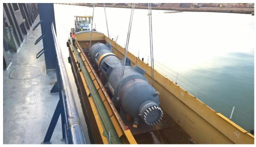
Road transports from Manufacturers to Porto Marghera and Taranto + Ocean transport to Novorossiysk, Russia (including direct discharge onto barge) of one complete Incinerator set (total abt 3500 cbm / 900 tons – including 1 x WHB 6.2 meters high weighting 110 tons) by chartering of suitable heavy lift geared vessel (Final Client: Afipskiy Refinery).
