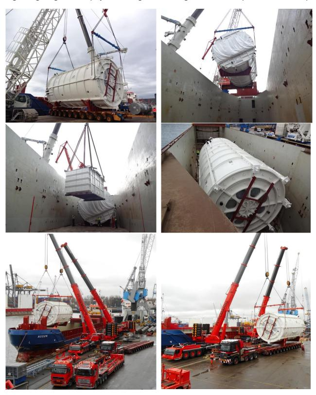
Loading (from shore and from barge) and ocean transportation of 3  $\times$  Reactors (weighting up to 140 tons each) from Porto Marghera to Marsa el Brega, Libya (Final Client: Lifeco).
