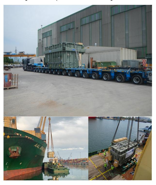
Sea-river transportation of 1 x Separator (measuring 19.5 x 5.0 x 5.5 m and weighting 193 tons) from Porto Marghera to Baku, by chartering of suitable sea-river vessel (Final Client: Bos Shelf).
