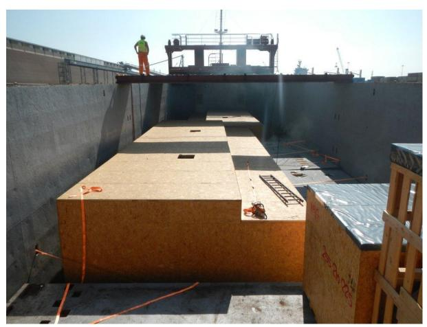
Road transport from Manufacturer up to Marina di Carrara port, loading onto Russian seariver vessel and lashing / securing / dunnaging / welding (including supply of suitable grillage for weight spreading purposes) of 3 Reactors measuring 25.6 x 4.4 x 5 meters each and weighting 206 tons each - Final client: Antipinsky Refinery.
