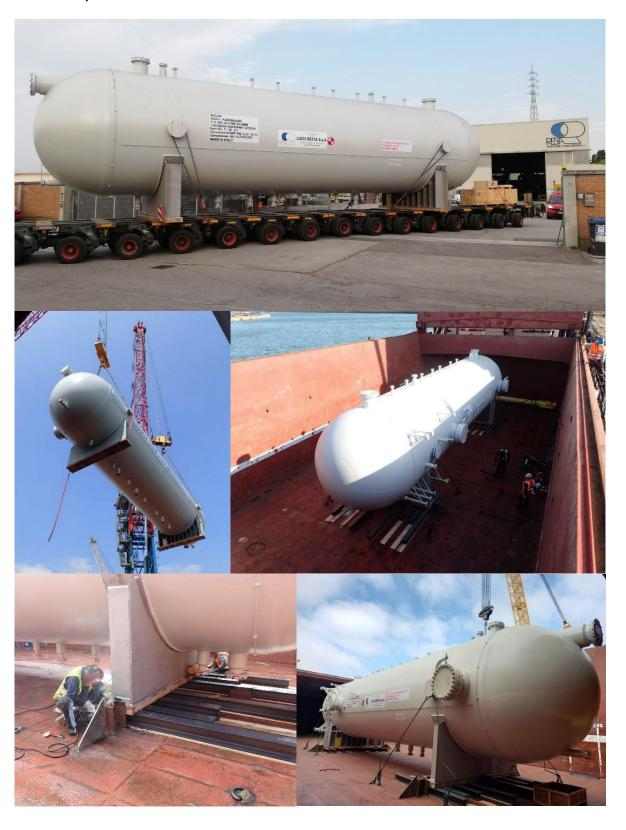
Multimodal transportation of 1 x Separator (measuring 18.5 x 4.8 x 5.8 m and weighting 95 tons) + 1 x Separator (measuring 11.0 x 4.9 x 5.8 m and weighting 77 tons) to Porto Marghera including road transport from Manufacturer to Valdaro river port, direct transshipment from trailers to barge and river transport from Valdaro to Porto Marghera.
