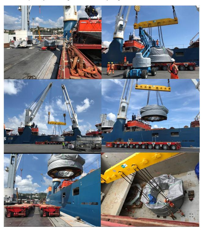
Multimodal transportation of 1 x Transformer weighting 158 tons (4.8 meters high) to Porto Marghera including road transport from Manufacturer to Valdaro river port, direct transshipment from trailer to barge, river transport from Valdaro to Porto Marghera.
