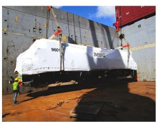
FAS Delivery + Loading Onto Vessel by mobile shore cranes + Sea Freight from Civitavecchia – ITALY to Botlek, Rotterdam – NETHERLANDS + Discharging onto quay by 2 floating cranes of 2 Columns dims mt 62,9 x 5,25 x 5,55 Weight 230 Tons + dims mt 41,7 x 4,67 x 4,9 Weight 93 Tons; Final Destination LYONDELL BASELL Chemical Plant.
