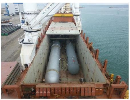
Ocean Transportation from Ulsan (South Korea) to Constanta (Romania) + discharging on pier + temporary storage + re-loading onto 4 Russian sea-river barges of total 9900 cbm / 1200 tons including nr. 6 large modules measuring up to 30 x 8 x 7 meters – 225 tons each + 1 reactor 42 x 4.5 x 5 meters – 170 tons. Final destination: Tuapse ROSNEFT Refinery.
