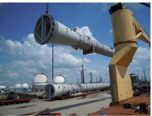
Sea freight of no.2 reactors dims mt 35,5 x 6,55 x 5,71 tons 401 + dims mt 26,6 x 4,95 x 5,63 tons 344 from Ortona Port to Kavkaz Port , Russian federation (discharged onto Russian heavy lift river barge; final destination Syzran Refinery) by chartering suitable heavy lift geared vessel (2 cranes WLL capacity 275 tons each, operating in twin-lift)
