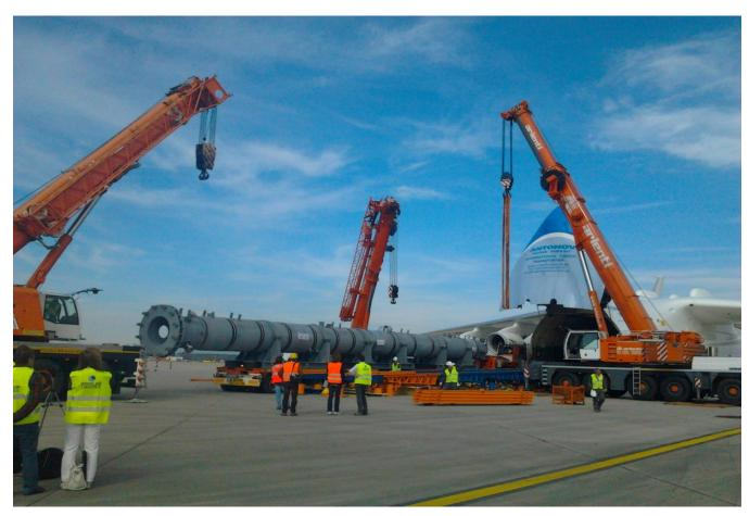
Loading operations have ended at **6.00pm on Saturday March 31st, 2012**. Just afterwards, lashing operations have started to fasten the items inside the hold. These operations were extremely important to comply with the ANTONOV standards that in this case require to contract with 2.5G of acceleration.
