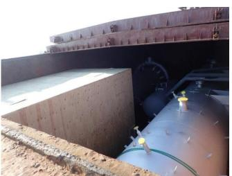
Road transport from Manufacturer to Porto Marghera + Ocean transport from Porto Marghera to Bandar Assaluyeh of nr. 2 x Steam Turbines weighting 180 tons each (5.1 meters high) by chartering of suitable heavy lift geared vessel.
