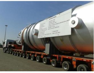
Sea freight of no.1 separator 1150 tons + nr. 1 Reactor 110 tons from Porto Marghera to St. Petersburg (discharged onto Russian heavy lift river barge; final destination TAIF-NK, Nizhnekamsk) by chartering suitable super heavy lift geared vessel (2 cranes WLL capacity 700 tons each, operating in twin-lift)
