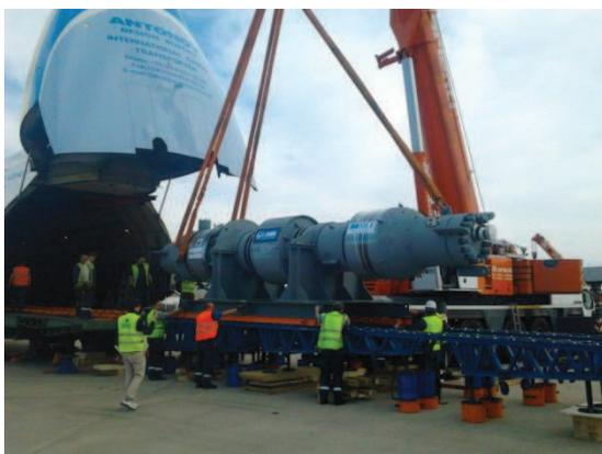
Loading operations of the Stripper and the Reactor have started at 3.30pm. 3x200t jib cranes have been working as a whole to load and position the items on the ramp with the utmost caution and accuracy. The plane winches have allowed the sliding of the items from the ramp to the final positioning into the AN-225 hold.
